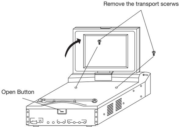
2. Push the monitor back into the monitor base unit until the screen engages with OPEN button. Then attach the brackets on both sides of unit with screws (M4x5), last install the unit with screws (M5x25). When fix the unit, you can slide the screw (M5x25) to left side or right side to meet your needed position. In the figure below, select two holes among the positions that marked 1, 2, 3 and 4 to fix the bracket.
