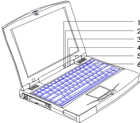
Two of these LEDs, Power and Standby, are visible even when you close the display cover so you can see the status of the computer while the cover is closed.
