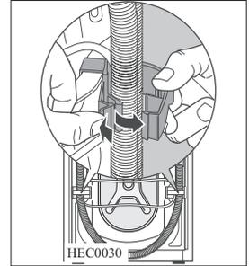
3. Unscrew the three bolts with the supplied spanner
