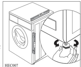
Carefully level by screwing the adjustable feet in or out. Never place cardboard, wood or similar materials under the machine to compensate for any unevenness in the floor.
