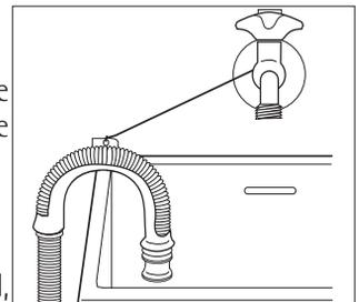
i.e. the inside diameter of the drain pipe must be larger than the outside diameter of the drain hose.
