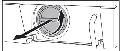
7. Remove any objects from the pump impeller by rotating it.
