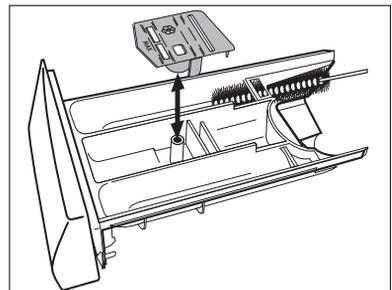
2. Remove the conditioner insert from the middle compartment.
