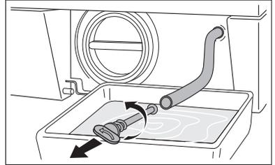
6. When no more water comes out, unscrew the pump and remove it. Always keep a rag nearby to dry up spillage of water when removing the pump.
