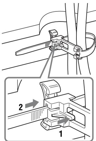
**To remove the cable tie from the rear of the stand**
