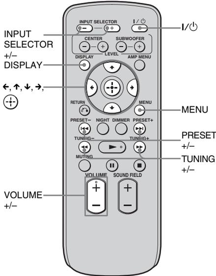
**1 Press INPUT SELECTOR + or - repeatedly until "FM" or "AM" appears in the front panel display.**
