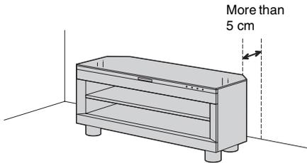
The stand has a back corner cut to fit in the corner of a room. If you install the stand in a corner of your room, it requires a space of about 86 cm from the corner of the room to the front of the stand.
