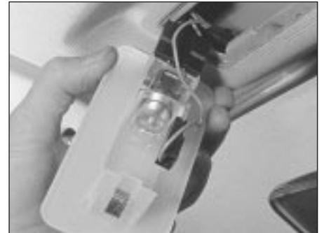
6.16b Interior (courtesy) light pivoted for access to the bulb
