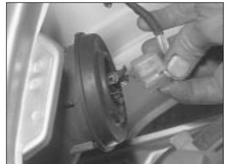
7.2 Disconnecting the multi-plug from the back of the headlight
