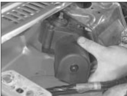
16.8b . . . and withdraw the wiper motor assembly
