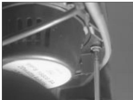
23.5a Remove the rear speaker securing screws . . .
