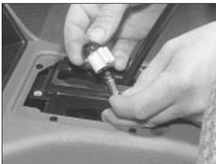
6.3a Remove the selector illumination bulb cover . . .
