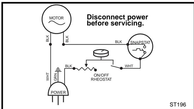
**Fig. 15** #2767 / FK26 Fan Wiring Diagram
