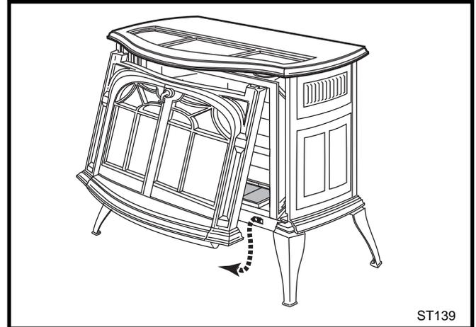
Fig. 36 Remove the front plate and top grille/screen.
