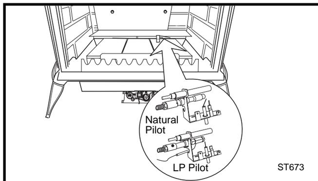
Fig. 30 Pilot assembly location.
