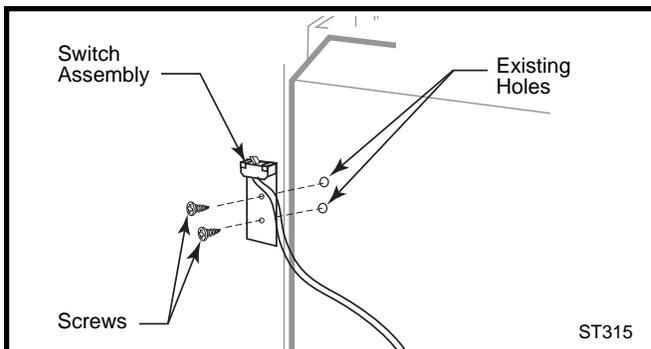
**Fig. 16** Attach switch assembly to rear shroud.
