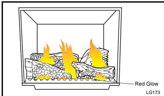
Fig. 33 Correct burner flame pattern.
