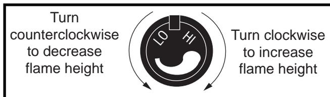
Fig. 31 Flame adjustment knob for Honeywell valve.
