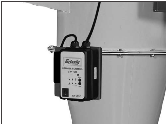
Figure 33. Switch mounted to funnel.
