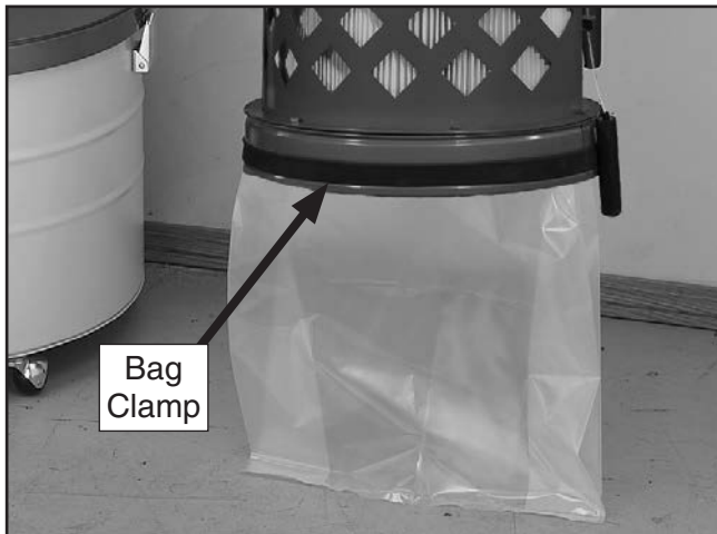
Figure 32. Plastic collection bag clamped in place under filter.
