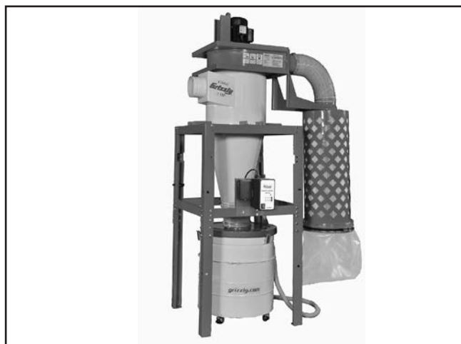
Figure 54. Cyclone mounted on stand.
