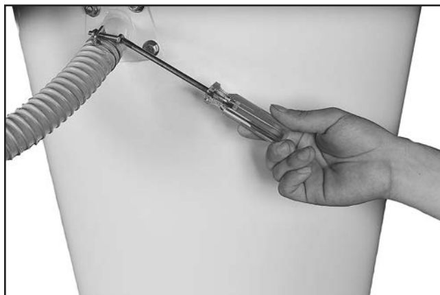
Figure 16. Cyclone vacuum tube and hose attachment.
