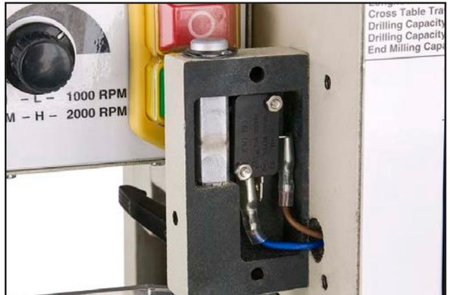
Figure 56. Guard limit switch.
