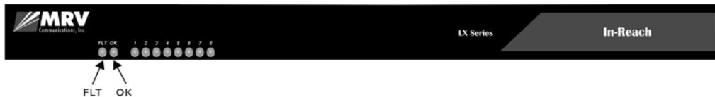
Figure 1 - LX Series 4008 Front Panel
