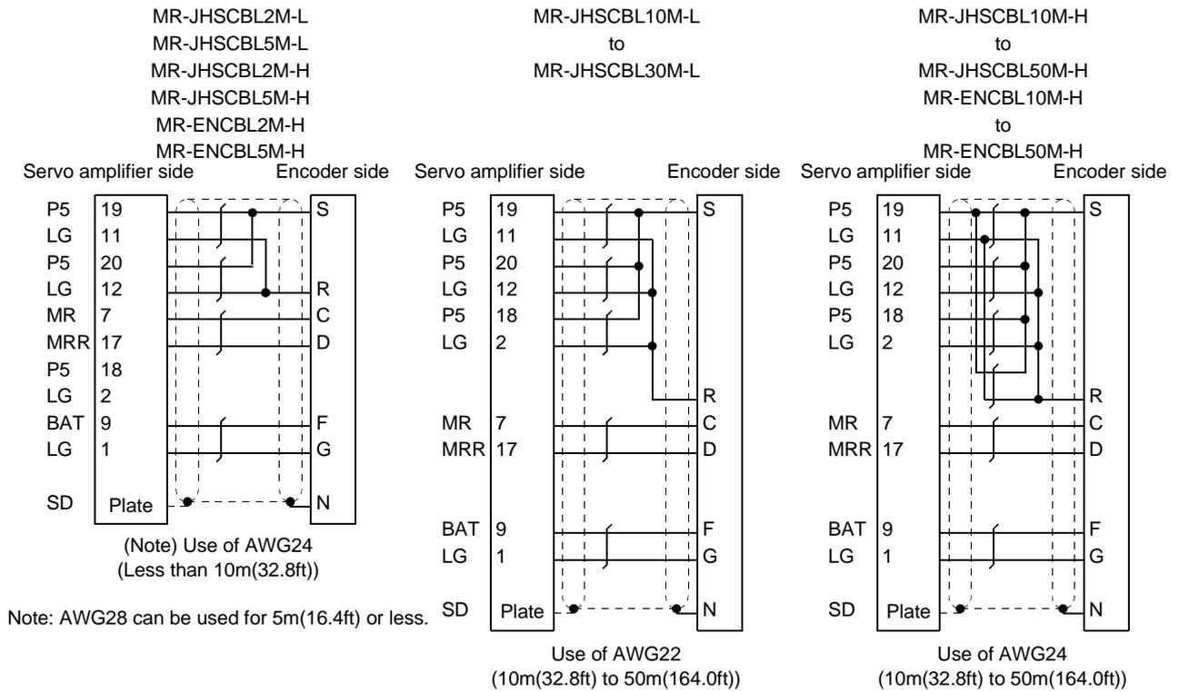
When fabricating an encoder cable, use the recommended wires given in Section 12.2.1 and the MR-J2CNS connector set for encoder cable fabrication, and fabricate an encoder cable in accordance with the optional encoder cable wiring diagram given in this section. You can fabricate an encoder cable of up to 50m(164.0ft) length. Refer to Chapter 3 of the servo motor instruction guide and choose the encode side connector according to the servo motor installation environment.
