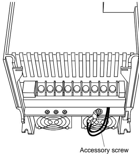
For the MR-RB51 install the cooling fan as shown.
