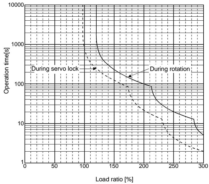
Fig 11.3 Electronic thermal relay protection characteristics 3
