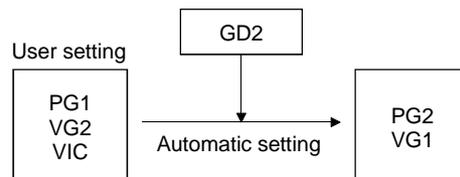
Therefore, you can adjust the model adaptive control system in the same image as the general PI control system (position gain, speed gain, speed integral time constant). Here, the position gain corresponds to PG1, the speed gain to VG2 and the speed integral time constant to VIC. When making gain adjustment in this mode, set the load inertia moment ratio (parameter No. 12) correctly.
