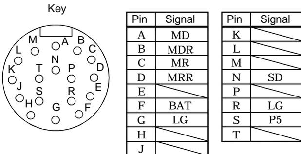
Electromagnetic brake connector signal arrangement
