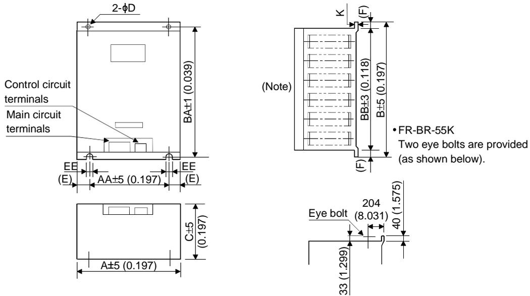
Note: Ventilation ports are provided in both side faces and top face. The bottom face is open.
