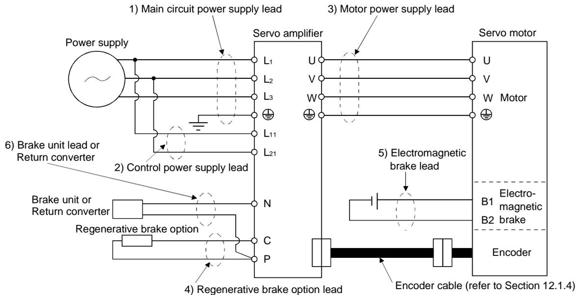
The following table lists wire sizes. The wires used assume that they are 600V vinyl wires and the wiring distance is 30m(98.4ft) max. If the wiring distance is over 30m(98.4ft), choose the wire size in consideration of voltage drop.
