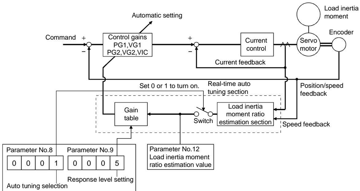
When a servo motor is accelerated/decelerated, the load inertia moment ratio estimation section always estimates the load inertia moment ratio from the current and speed of the servo motor. The results of estimation are written to parameter No. 12 (load inertia moment ratio). These results can be confirmed on the status display screen of the servo configuration software section.
