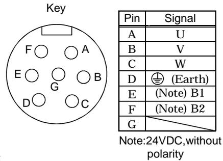
Encoder connector signal arrangement
