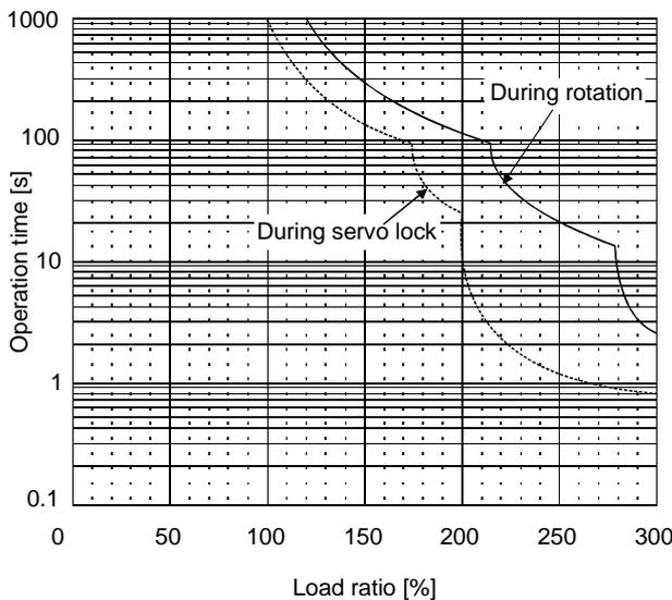
Fig 11.2 Electronic thermal relay protection characteristics 2
