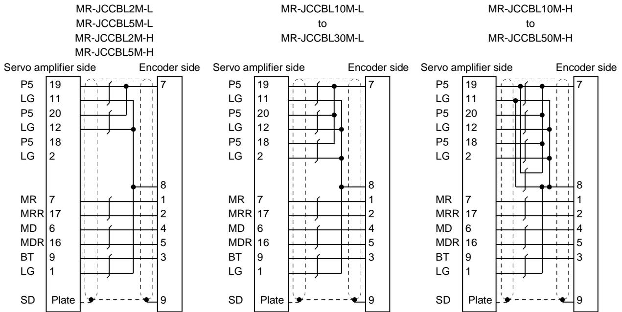
When fabricating an encoder cable, use the recommended wires given in Section 12.2.1 and the MR-J2CNM connector set for encoder cable fabrication, and fabricate an encoder cable as shown in the following wiring diagram. Referring to this wiring diagram, you can fabricate an encoder cable of up to 50m(164.0ft) length including the length of the encoder cable supplied to the servo motor.
