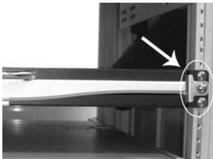
2. Attach the extensions (from the Rear bracket & extension kit) to both sides of the KVM switch module. Please note the length of the extensions and mount them as shown. For a 2U module, the extensions are mounted to the lower half of the module.
