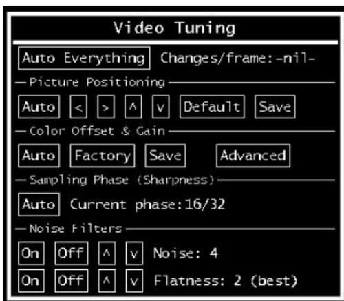
Use the Auto Everything button to automatically fine-tune all three adjustments. If the test pattern for Color Offset calibration is not present on the screen, then the Color Offset adjustment is skipped.
