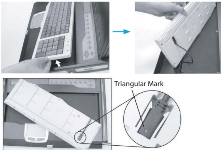
**NOTE:** There is a round hole under the drawer, which can be used to pass one finger through allowing for easier removal of the keyboard (pushing upwards). The triangular mark on the mini USB connector must face outwards.
