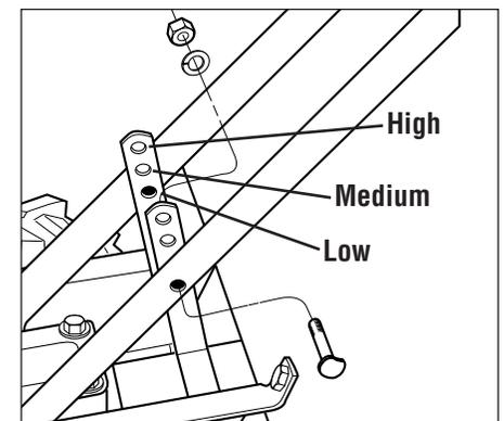
Figure 3-6: Handlebar height adjustment.
