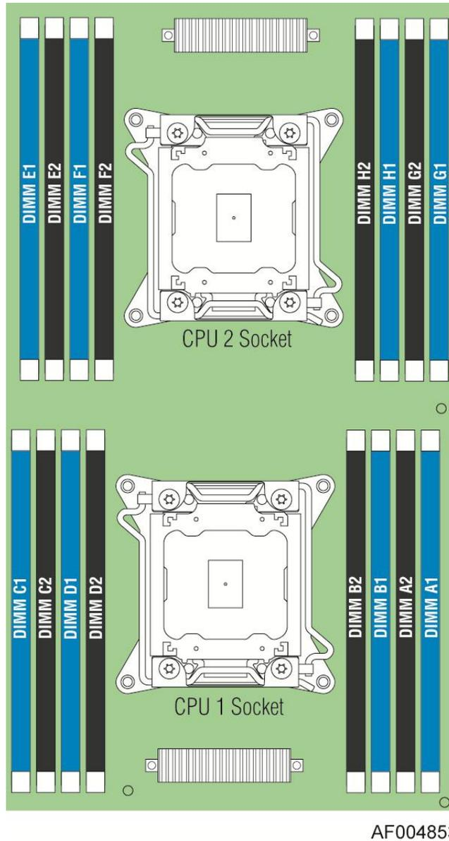
**Figure 6. DIMM Slot Order**
