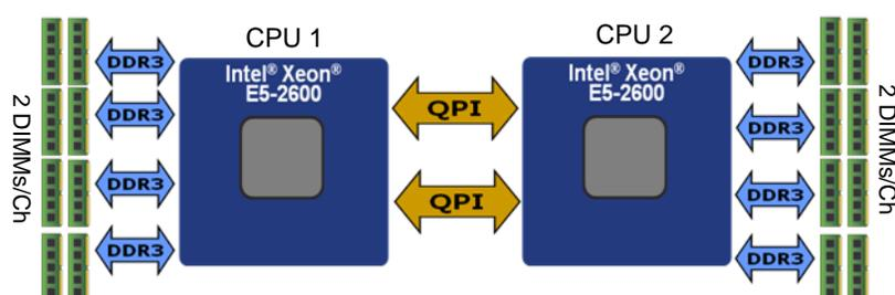
**Figure 5. Intergrated Memory Controller (IMC) and Memory Subsystem**
