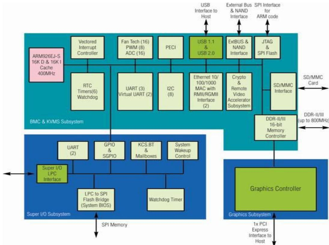
Figure 7. Integrated BMC Functional Block Diagram
