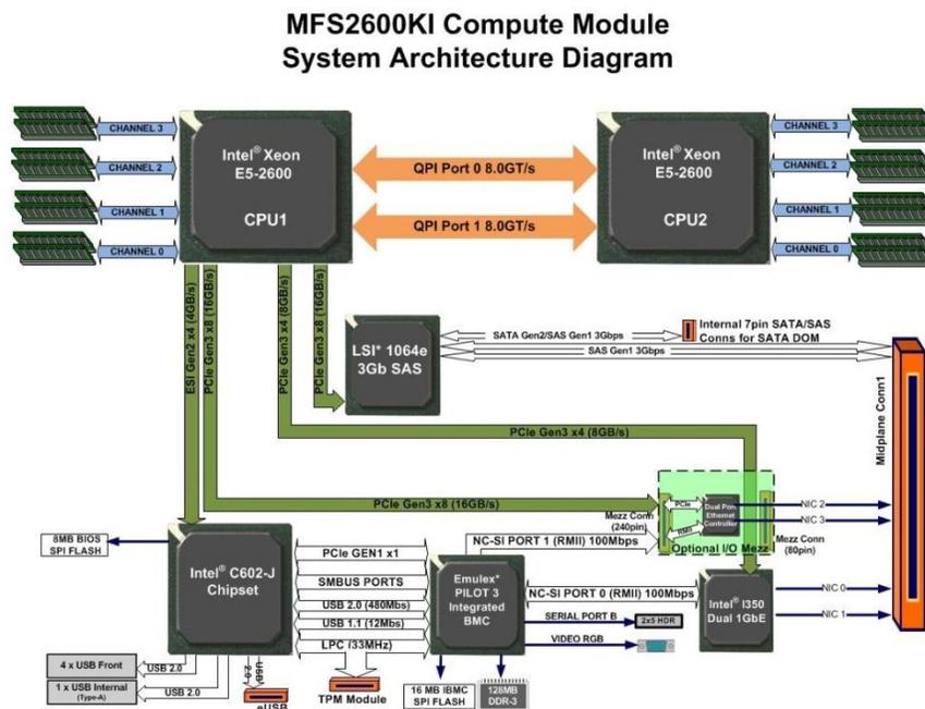
Figure 3. Intel® Compute Module MFS2600KI Functional Block Diagram
