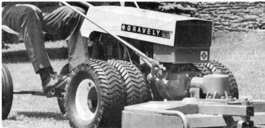
40" COMMERCIAL MOWER ATTACHED TO C12 TRACTOR WITH DUAL WHEELS
