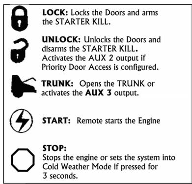
Pressing the **LOCK** and **UNLOCK** buttons simultaneously will activate the **AUX 2** output.
