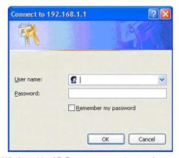
In order to configure the Wireless 11g AP Router, you must enter the password into the **Password** box and leave the **User Name** blank. The default password is "admin".
