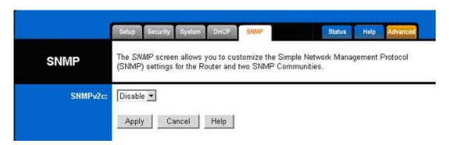
**SNMP:** The SNMP screen allows you to customize the Simple Network Management Protocol (SNMP) settings. SNMP is a popular network monitoring and management protocol.
