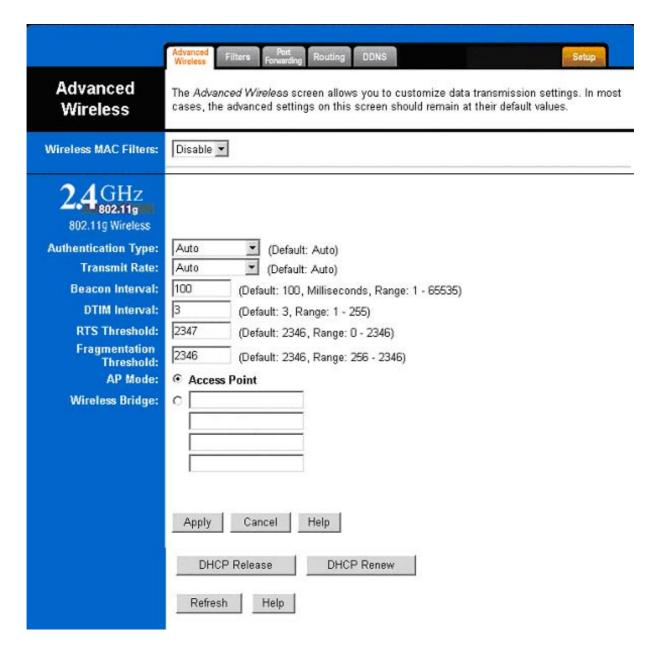
**Wireless MAC Filters:** This function allows the administrator to have access control by entering MAC addresses of client stations. When this function has been **Enabled**, two new options will appear.
