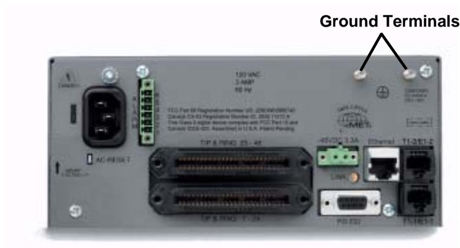
1. Route wire (#6 or #8 AWG copper) from building ground to lug on Unit.
