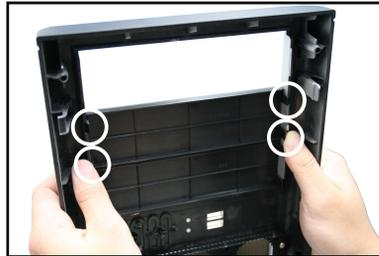
3. Unscrew and remove the metal cover of the bay where you want to install the 5.25-inch drive
