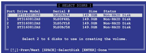
5. Use the up/down arrow keys to select a drive, and then press <Space> to select. A small triangle marks the selected drive. Press <Enter> after completing your selection.
