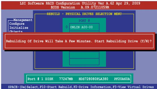
4. When rebuild is complete, press any key to continue.
