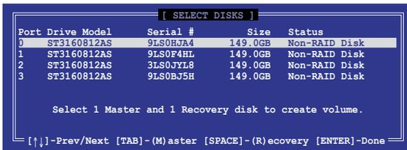
5. Use the up/down arrow keys to select a drive, press <TAB> to select a Master disk, and then press <SPACE> to select a Recovery disk. A small triangle marks the selected drive. Press <Enter> after completing your selection.
