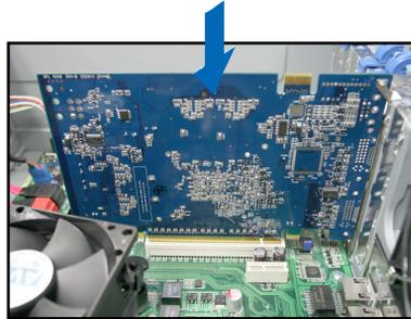
7. Restore the expansion card lock to its original position. A light click indicates that the card is locked in place.
