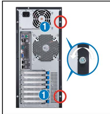
2. Slide the side cover for about half an inch toward the rear until it is disengaged from the chassis.
