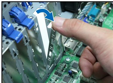
6. Align the card golden fingers with the slot, and then press firmly until the card is completely seated on the slot.
