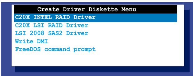
5. Use the arrow keys to select the type of RAID driver disk you want to create and press <Enter> to enter the sub-menu.
