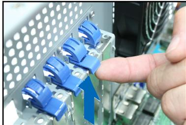
5. Remove the metal slot cover opposite the slot where you wish to install an expansion card.
