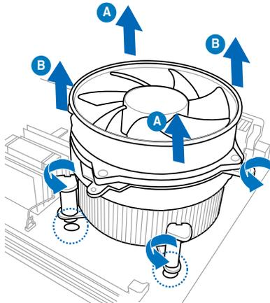
4. Carefully remove the heatsink and fan assembly from the motherboard.
