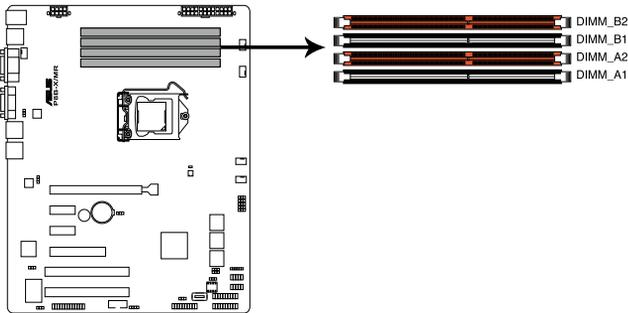
**P8B-X/MR 240-pin DDR3 DIMM sockets**
