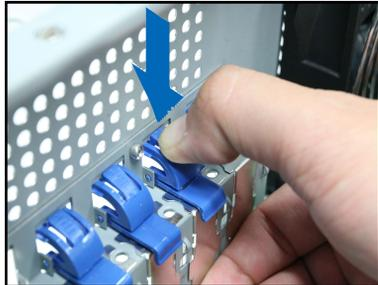
4. Lift up the expansion card lock as shown.
