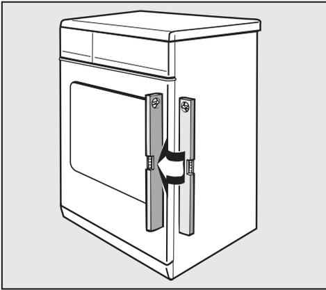
The machine must be perfectly level to ensure safe and proper operation.
