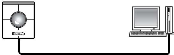
Ethernet cable (Category 5 cross cable)
