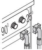
Connect the special water supply hoses supplied with the product to the water inlets on the product. Red hose (left) (max. 90 °C) is for hot water inlet, blue hose (right) (max. 25 °C) is for cold water inlet.
