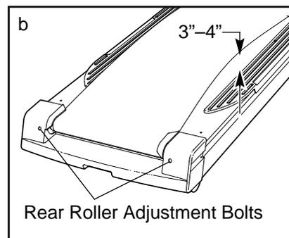
**PROBLEM****SOLUTION****4. The walking belt is off-center or slips when walked on**
