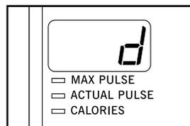
when a treadmill is displayed in a store. When the console is in the demo mode, the power cord can be plugged in, the key can be removed from the console, and the displays and indicators on the console will automatically light in a preset sequence, although the buttons on the console will not operate. **If a “d” appears in the Pulse/Calories display when the information mode is selected, press the Speed – button so the Pulse/Calories display is blank.**
