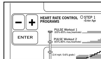
The profiles on the console show how the target heart rate will change during the programs. The program display will show a simplified profile of the program. The Time/Segment Time display will show how long the selected program will last.
