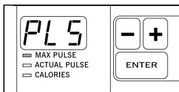
Press the + or – button. A number will then appear in the display. This number is the maximum heart rate setting for the program. If Pulse program 1 is selected, the maximum heart rate setting can be from 65% to 85% of your maximum possible heart rate; if Pulse program 2 is selected, the maximum heart rate setting can be from 65% to 80% of your maximum possible heart rate.
