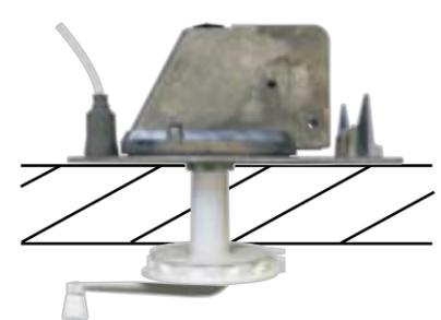
**NOTE** The set screw simply holds the elevating crank to the rotating base shaft.
