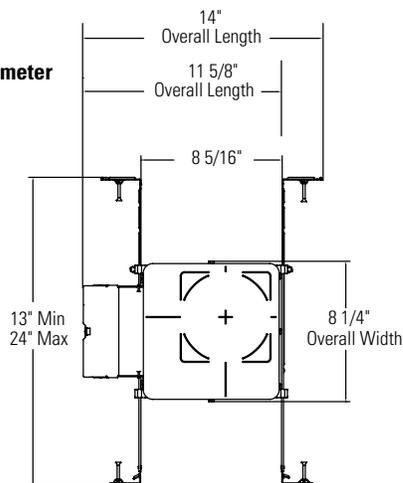
Complete Fixture consists of Frame-In Kit and Reflector Trim. Select each separately.
