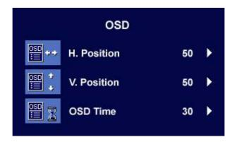
Press ◀ or ▶ key to adjust the Horizontal Position of the OSD, press "Exit" to return to previous menu.
