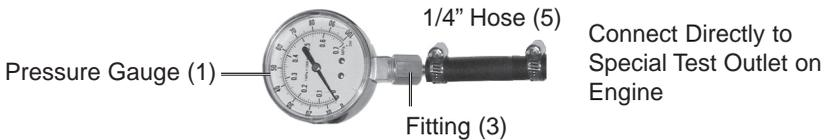
Screw on Female Swivel Coupling to Engine Test Fitting
