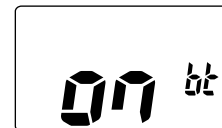
Battery voltage indication ON
