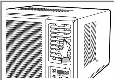
*The outer air flow blades can be adjusted to control the vertical air flow direction.*
