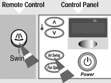
*Depending on the position of the unit in your room, you can adjust the orientation of the inner air flow blades on the right-hand side of the unit, thus increasing the efficiency of the air conditioner.*
