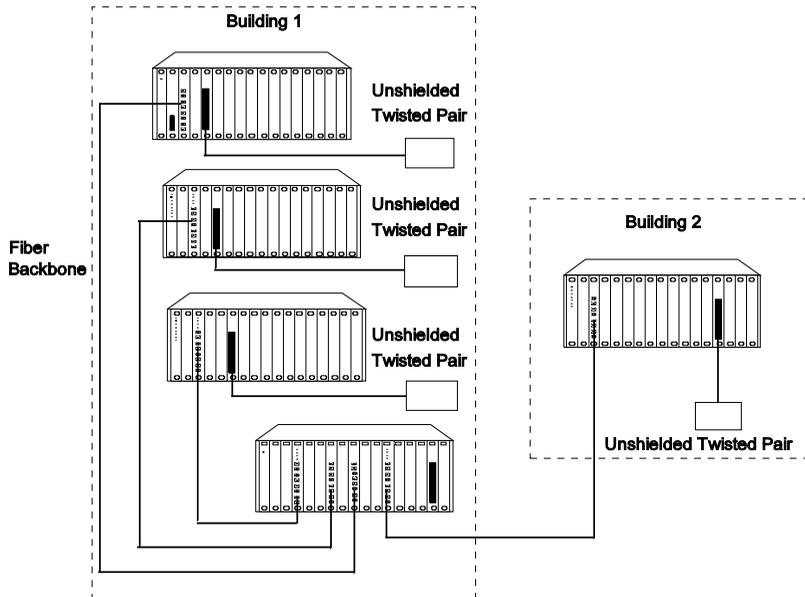
**Figure 2-3. Star-Wiring Configuration**
