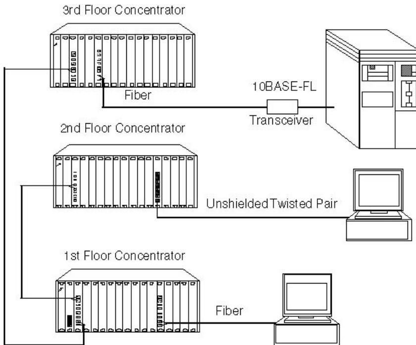
**Figure 1-1. 10BASE-FL Module Connections**
