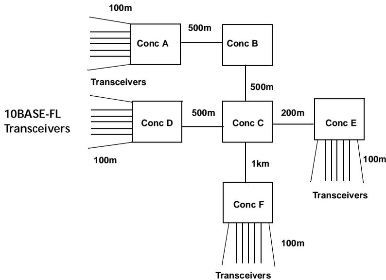
**Note:** All 10BASE-FL Transceiver connections to concentrators (each populated with 10BASE-FL Modules) are 100 meters of fiber.
