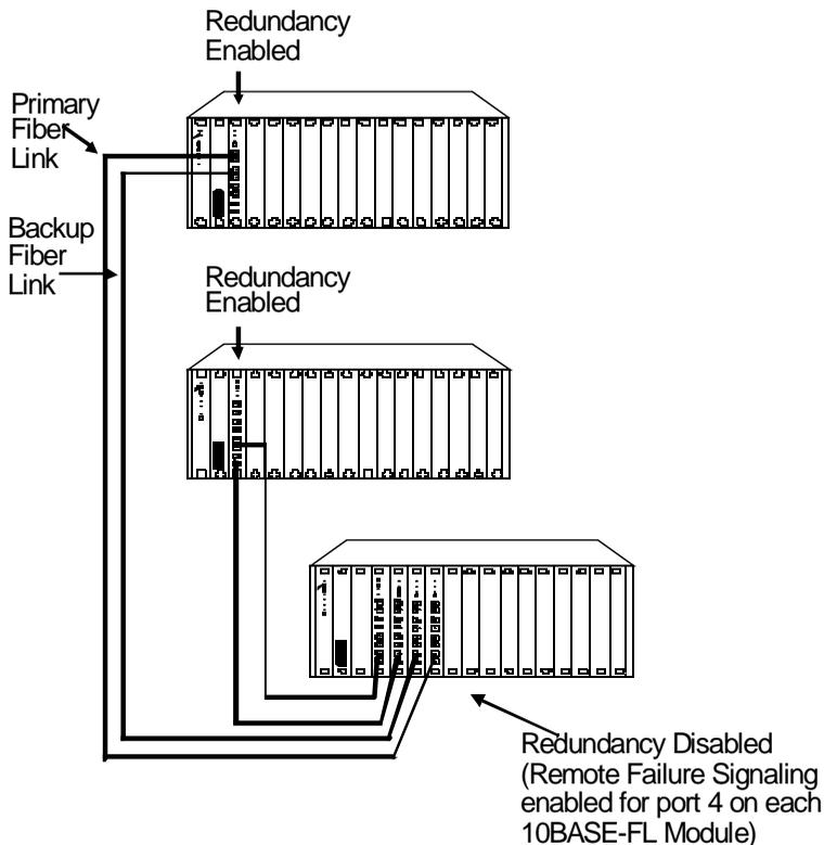
**Figure 2-11. Total Backbone Fault-Tolerant Configuration**
