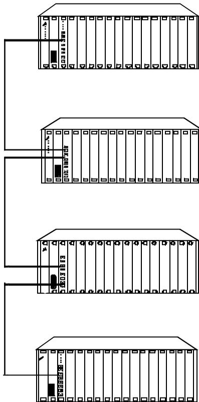
*Figure 2-4. Serial Configuration Using 10BASE-FL Modules*
