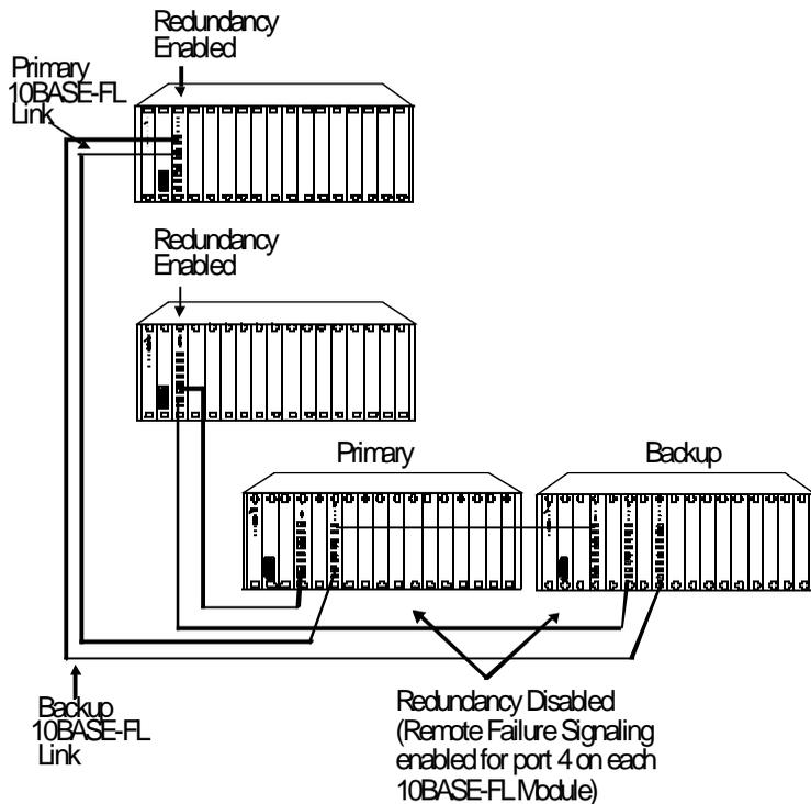
**Figure 2-10. Redundant Fiber Backbone Configuration**
