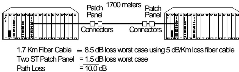
**Figure 2-2. 1700 Meter Fiber Link Through Two Patch Panels**
