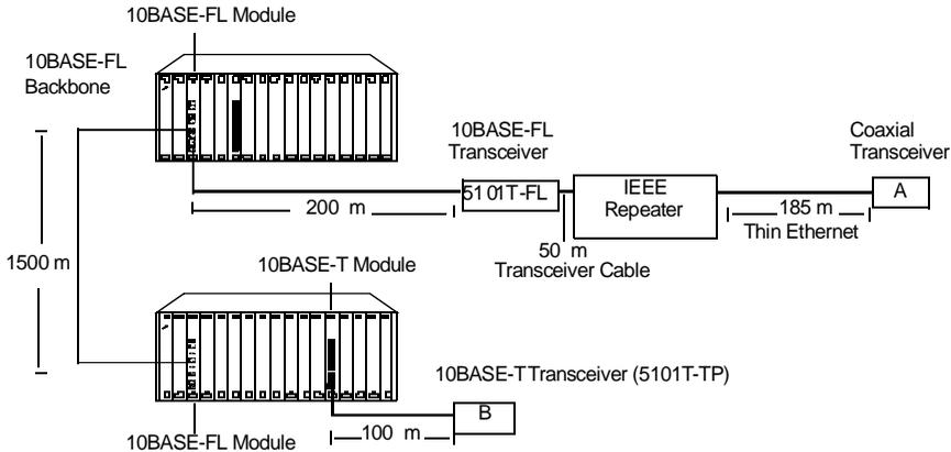
**Figure 2-9. Thin Ethernet Segment Connecting to ONline Using an IEEE Repeater**
