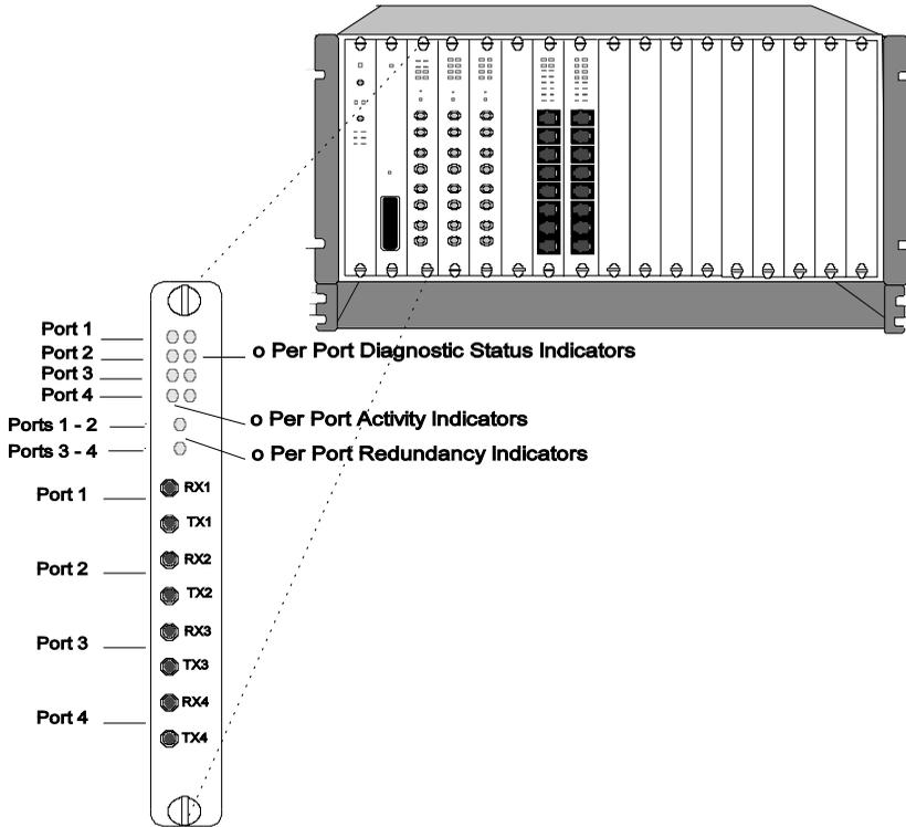
**Figure 3-5. 10BASE-FL Module Faceplate and ONline System Concentrator**
