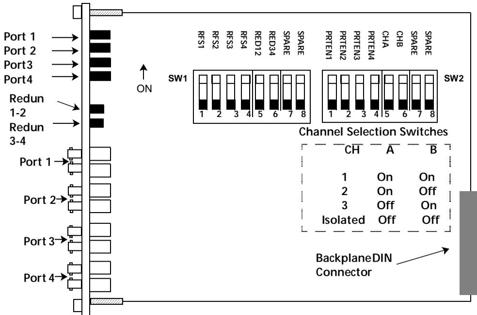
**Figure 3-1. 10BASE-FL Module Dip Switch Locations**
