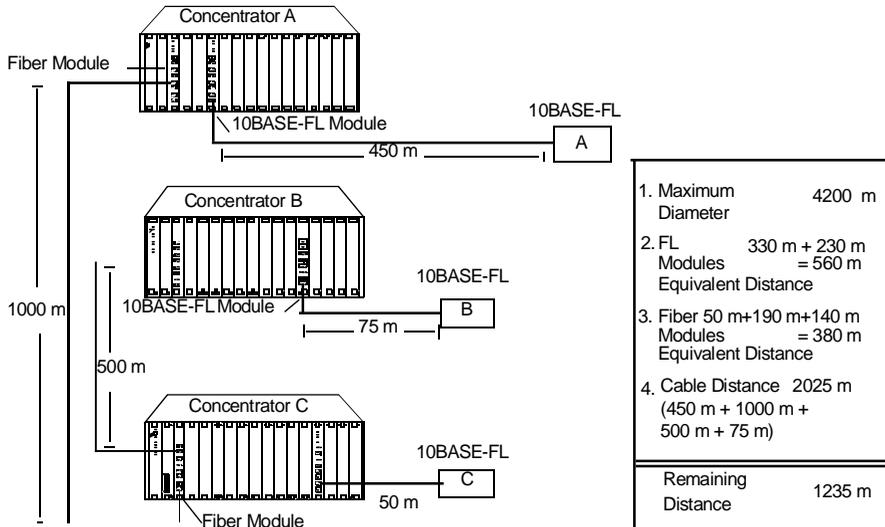
**Figure 2-8. Sample Fiber Backbone, 10BASE-FL to-the-Desk Configuration**
