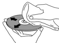
Wipe lightly from the center of the disc using straight strokes.
