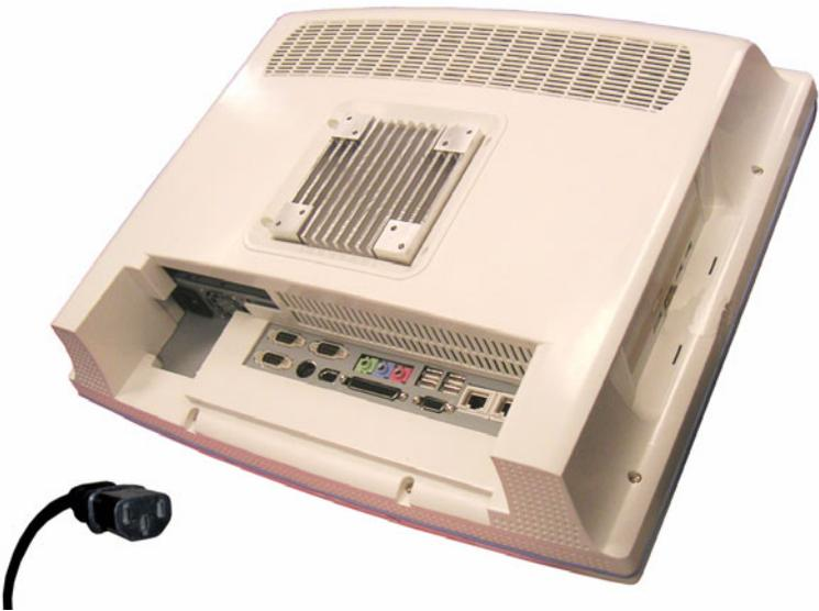
*Figure 2.4: Connecting the power cord*
