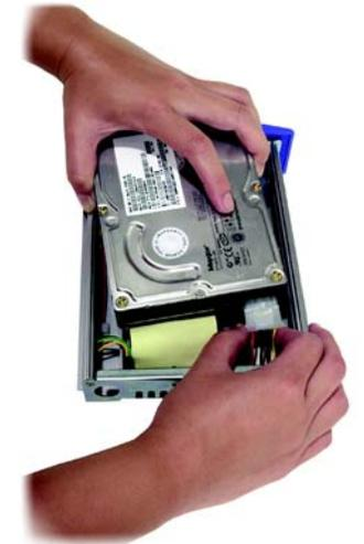
Figure B-2: Attach Power Cable
