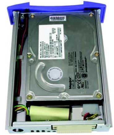
**Figure B-3: Make Sure Connections are Tight**
