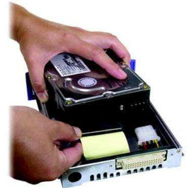
Figure B-1: Attach IDE Cable
