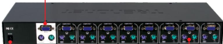
3. Connect the included AC Power Adapter to the KVM switch and then to a power outlet (TK-801R /TK-1601R only).
