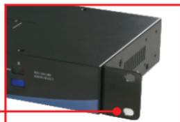
2. Carefully position the KVM switch onto the rack. Align the bracket to the screw holes on the rack, then use the screws provided with the equipment rack to mount the KVM switch.
