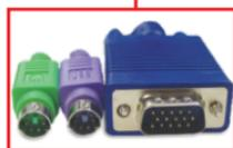
4. Use the PS/2 KVM cables to connect your PC to the KVM switch.
