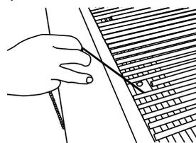
5. Push in and turn the burner knob to LITE/HI for the burner closest to the lit match. The burner will light immediately. When burner is lit, turn knob to desired setting.
