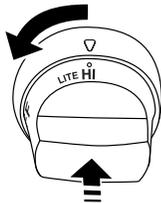
**IMPORTANT:** If the rotisserie burner does not light immediately, turn the rotisserie burner control knob to “OFF” and wait 5 minutes before relighting.
