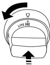
4. You will see the igniter glow. When burner is lit, release the knob. Turn knob to desired setting.
