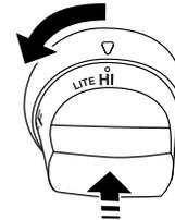
3. When the rotisserie burner lights, continue to hold the knob in for another 10 seconds, then release the knob and burner will stay lit.
