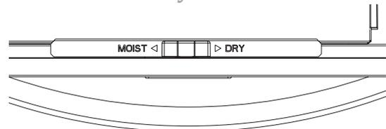
The Moist-Dry slide control allows you to open or close the vent slots in the door. The MOIST setting holds moisture in, while the DRY setting allows steam and moisture to escape from the drawer.
