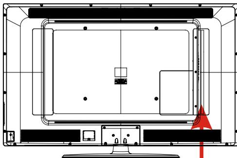
1. AC IN and POWER SWITCH: Main power input.
