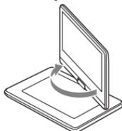
After rotating the LCD panel 180 degrees clockwise, push the LCD panel down onto the main body of the player. In this position the panel is facing up.
