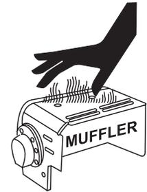
■ The engine section of this generators requires an adequate free flow of cooling air. **NEVER** operate the generators in any enclosed or narrow area where free flow of the air is restricted. If the air flow is restricted it will cause serious damage to the generators or engine and may cause injury to people. Remember the generator's engine gives off **DEADLY** carbon monoxide gas.
