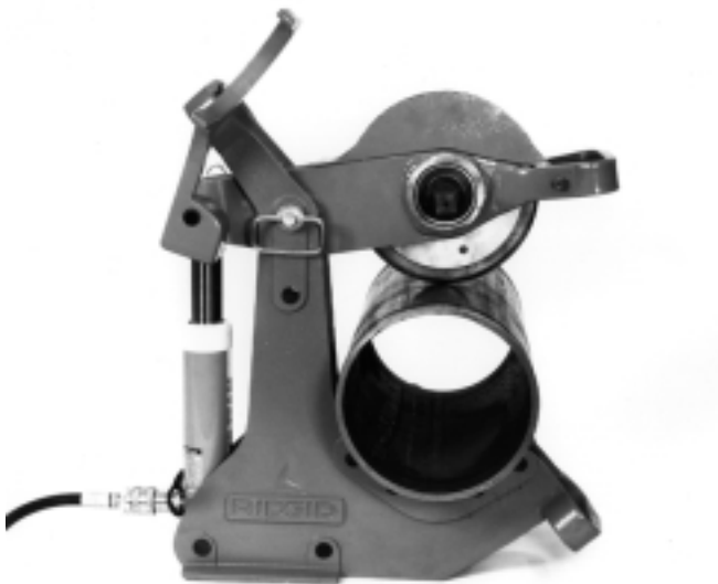
Figure 8 – Positioning Pipe in Cutter
