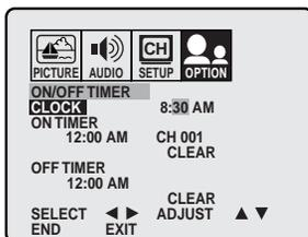
6. Press ▲ or ▼ to set the minutes, then press EXIT to return to normal viewing.
