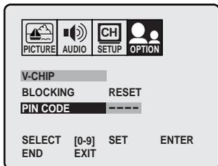
4. Use the Channel Number buttons (0–9) to enter your PIN code. If you are accessing the V-Chip menus for the first time, select a four-digit number to be your PIN code. Press ENTER. The BLOCKING menu appears.
