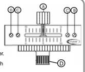
◆ Your Gemini mixer comes with an RG-45 PRO (RAIL GLIDE™) DUAL-RAIL CROSSFADER. Rail Glide™ Crossfaders have internal dual stainless steel rails that allow the slider to ride smoothly and accurately from end to end.
