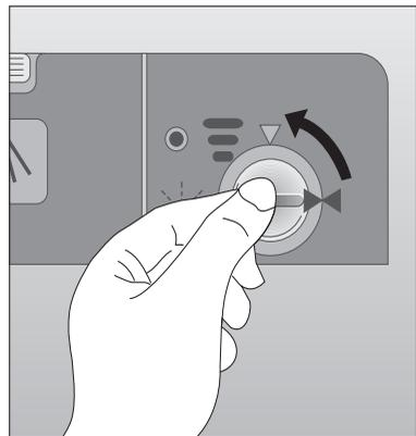
3. Fill with rinse aid, up to the broken line (maximum); this line corresponds to a quantity of approx. 150 ml
