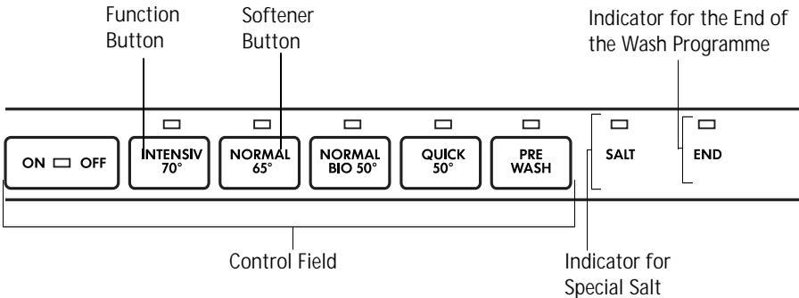
The **Control Field** comprises the On/Off switch
