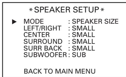
This menu allows you to switch the menu to change either the speaker size setting or the exact crossover point used for that speaker group. For the first pass through the menu, leave the setting at its default option of SPEAKER SIZE, and then proceed as outlined below. Once the speaker choices have been set, you may wish to return to this line to change the option so that the crossover settings may be adjusted.
