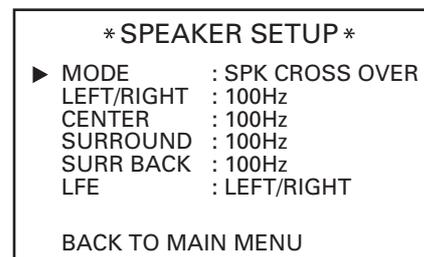
The factory default setting for all speaker positions is 100Hz. If that setting is acceptable for all channels, then no adjustments are needed and you may skip this section. However, should you wish to change one of the settings. The available choices at which point low-frequency information will be sent to the subwoofer, rather than to the main speaker channel, are 40Hz, 60Hz, 80Hz, 100Hz, 120Hz and 200Hz.
