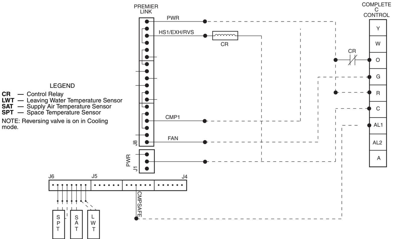
**Fig. 7 — PremierLink Controller Applications with Complete C Control**
