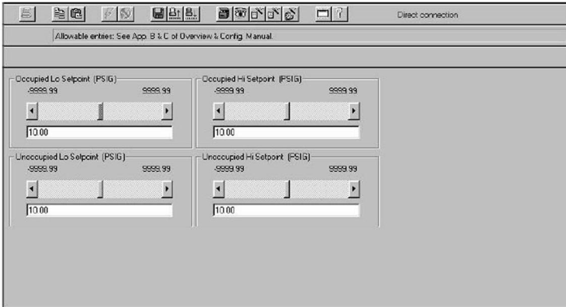
**Fig. 12 — System Pressure Set Point Screen**
