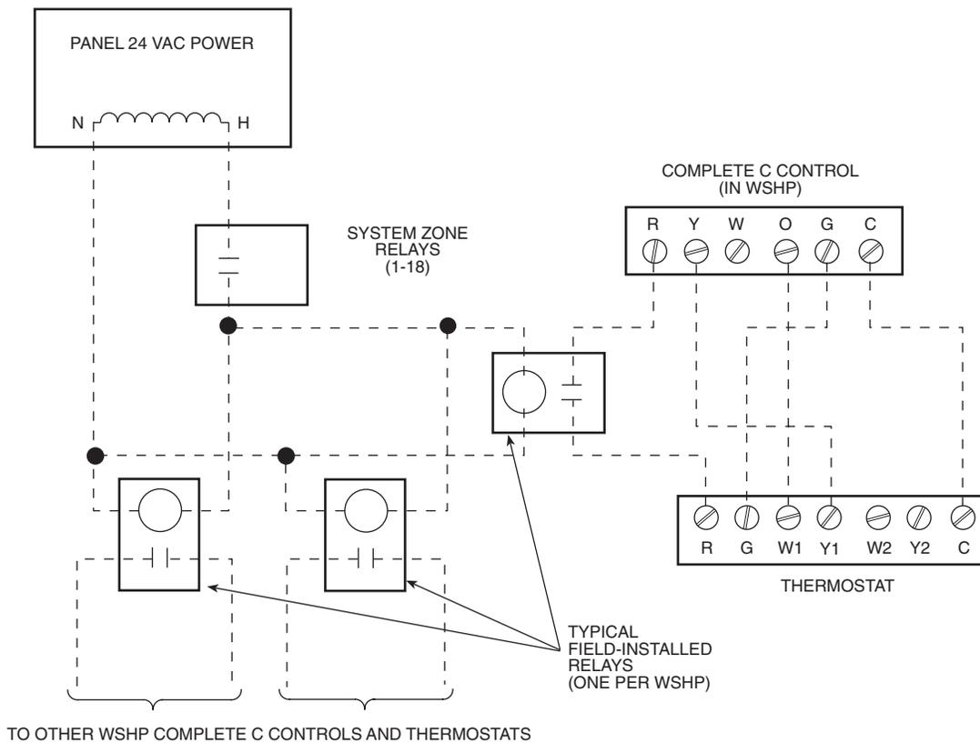
**Fig. 5B — System Zone Relay Wiring (Aquazone System Control Panel Used to Control Multiple Thermostats)**
