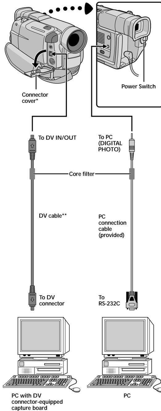
\* When connecting the cable, open this cover.
