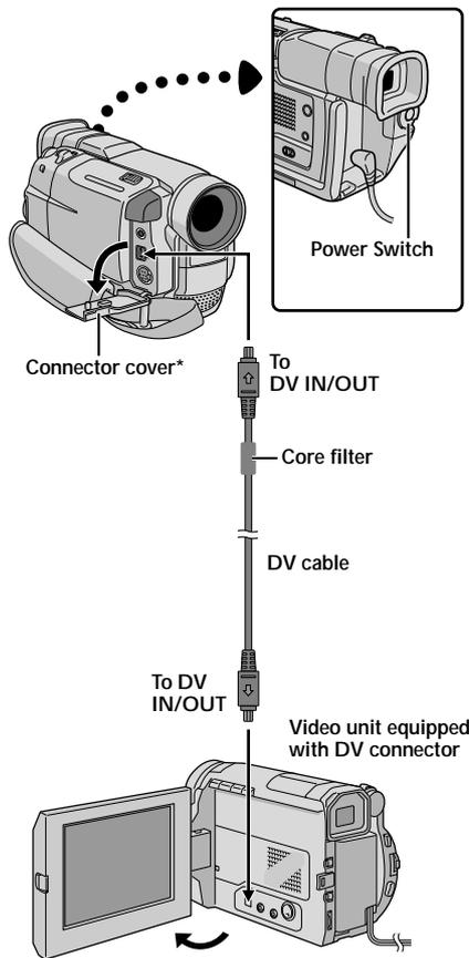
\* When connecting the cable, open this cover.
