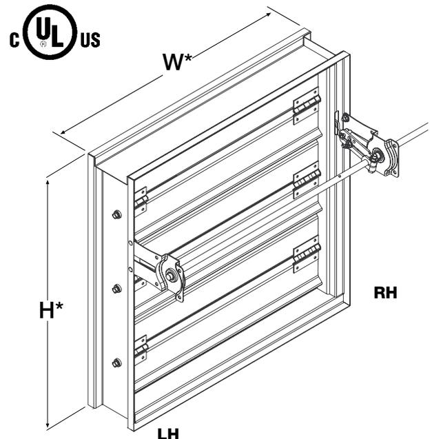
\*W & H dimensions furnished approximately 1/4 in. (6mm) undersize. (Add sleeve thickness for overall sleeved damper dimension)
