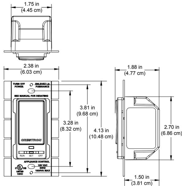
The -SW4RF and -SWS4RF have a light emitting diode (LED) with adjustable brightness (via Crestron programming software), four pushbuttons, and a three-position mode selection switch as shown in the following diagrams. Each of the buttons may be pushed to perform certain functions. The function of each pushbutton is determined by the position of the mode selection switch. For more information, refer to “Operation” on page 9.
