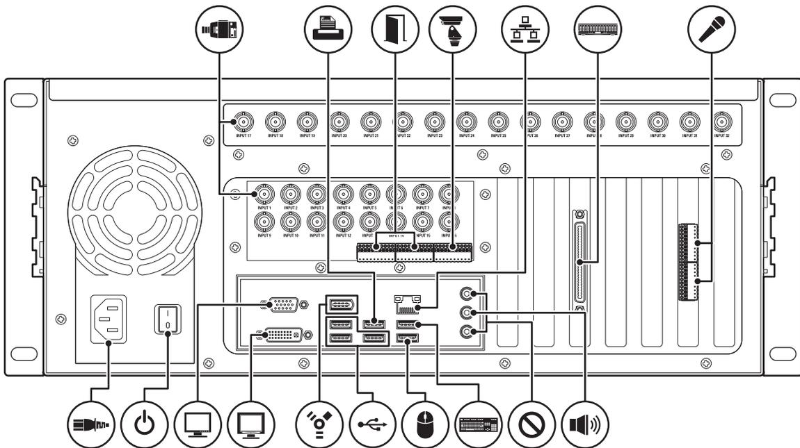
**NOTE:** The top row of video input BNCs (inputs 17-32) is available only on 32-input systems. The SCSI connector for RAID storage is optional.
