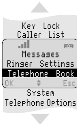
Selection lists (e.g. telephone book) and the features menu are shown in the display as a three-line excerpt. Using the arrow key, the lines of text can be scrolled up or down. A selectable entry is shown inversely, with a dark background.
