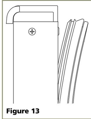
3. Pull door gasket out of groove (top edge of door only). Start in the middle and pull outward, moving toward the edge (see **Figure 13**). This may take some force. Do not remove the three screws behind gasket.
