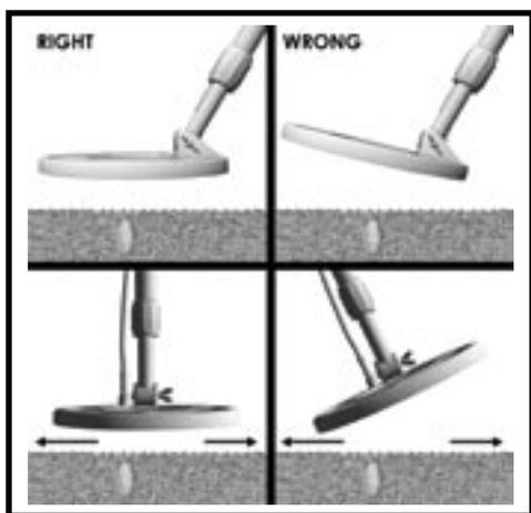
Figure 5. "sweeping" the search coil. Keep the search coil parallel and close to the ground at all times
