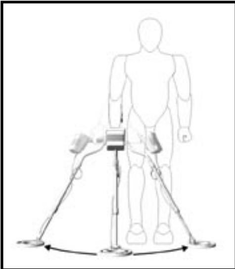
When the stem length is properly adjusted, the 1225-X is balanced for sweeping in a tight semicircle. Always overlap your sweeps by at least 50% or you'll miss a lot of the deeper targets.
